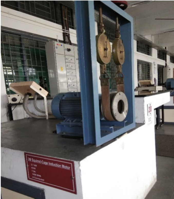
Fig. 2 Testing equipment to conduct load test on three-phase 5 HP induction motor
