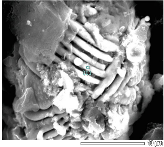
Fig. 8 Pellet with 30% LECO reduced at 1200 °C
