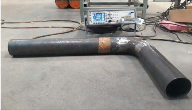
Fig. 5 Arrangement of mild steel pipe specimen with LCR meter
